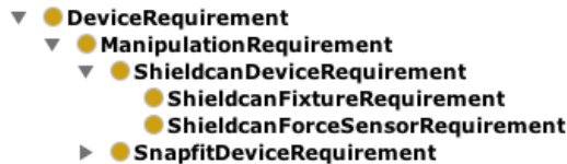
Figure 11: The device requirements of the skill ShieldCanInsertion are modelled in an ontology. The ManipulationRequirement which several skills inherit from, is that a gripper has to be mounted on the robot. The ShieldcanFixtureRequirement and the ShieldcanForceSensorRequirement list that there must exist a fixture and a force sensor that have to be vertically aligned (not shown in the picture).
