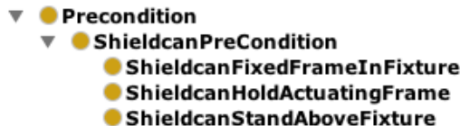
Figure 12: There are three preconditions to the ShieldCanInsertion skill. The skill has two feature frames (relative coordinate frames) as input parameters, where one is a reference object frame and the other is attached to the object in the gripper, i.e., an actuating frame. The first precondition is that the object with the reference frame has to be on the fixture. Secondly, the object with the actuating frame should be attached to the gripper, see Fig. 13, and finally, the position of the actuating object should be above the fixture. Imprecise geometrical relations such as “Above” are given concrete values by the Engineering System.
