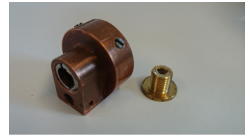
Figure 5.4. The copper mount for the laser diode and the collimation lens glued into a brass mount.
