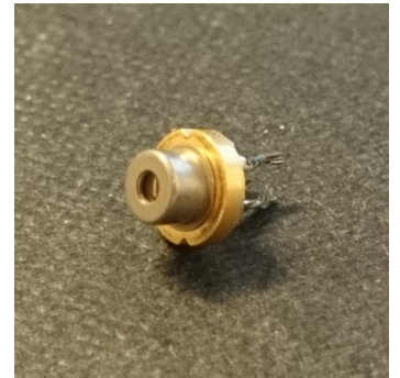
Figure 5.1. The Toptica LD-0375-0020-2 laser diode.
