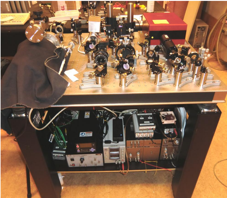
Figure 5.15. The 370 nm laser stabilization system. Both the optics and the electronics are placed on a table with wheels.
