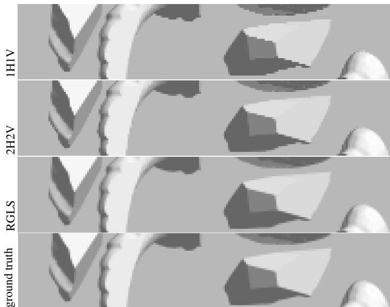
Figure 10: Here we compare the line sampling pattern quality for a static frame of the breaking armadillo. As can be seen, rotated grid line sampling (RGLS) is substantially closer to the ground truth (256 stochastic samples) than the other two.
