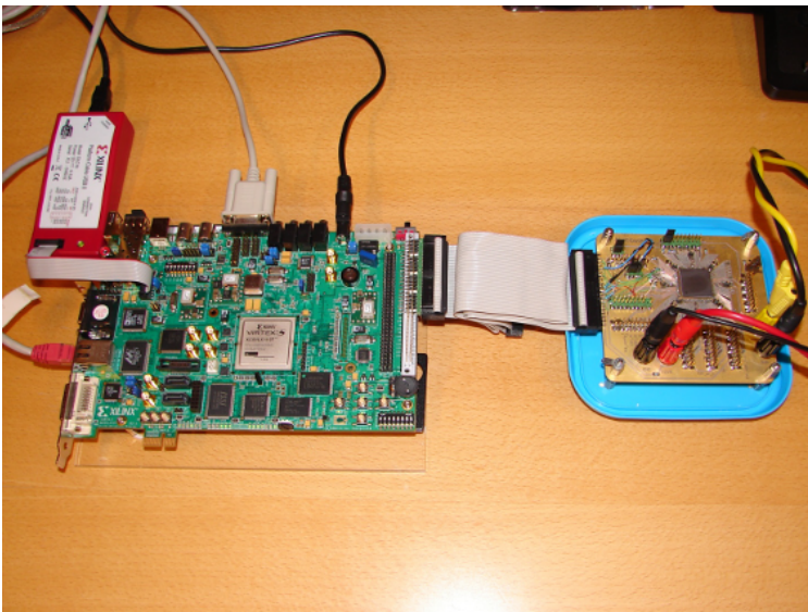
Figure 14.4.: Synchronization engine stand-alone verification setup, communication is done via serial interface under lower operational frequency and communicated to computer via serial port.
