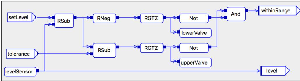
**Figure 11.** Simple tank regulator in Bloqqi. The block levelSensor reads the current liquid level. The blocks lowerValve and upperValve are actuators to the valves. The block RGTZ means greater than zero (for reals).
