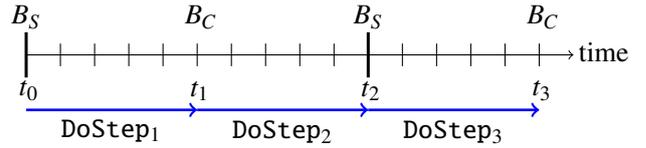
**Figure 8.** The execution starts when the simulated time has passed the value of the variable starts. This means that the first and third invocation of DoStep will start an execution, but not the second invocation. The second invocation is between the times  $t_1$  and  $t_2$ , but it has not passed  $t_2$ , which is required for it to start executing.
