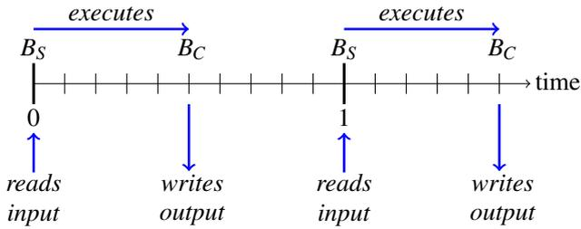
**Figure 6.** Simulation of a Bloqqi FMU with sampling period of 1 second and execution time of 0.5 seconds. The Bloqqi program starts executing at  $B_S$  and completes at  $B_C$ . The inputs are read at  $B_S$  and the outputs are set at  $B_C$ . The time on the axis is the simulated time.
