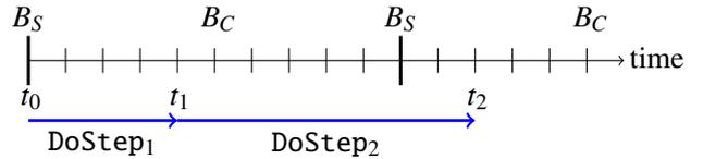
**Figure 9.** When the master algorithm makes the second call to DoStep in this example, the Bloqqi FMU should first write outputs from the previous execution before starting a new execution. This is handled by checking the variable completes before starting a new execution in DoStep.
