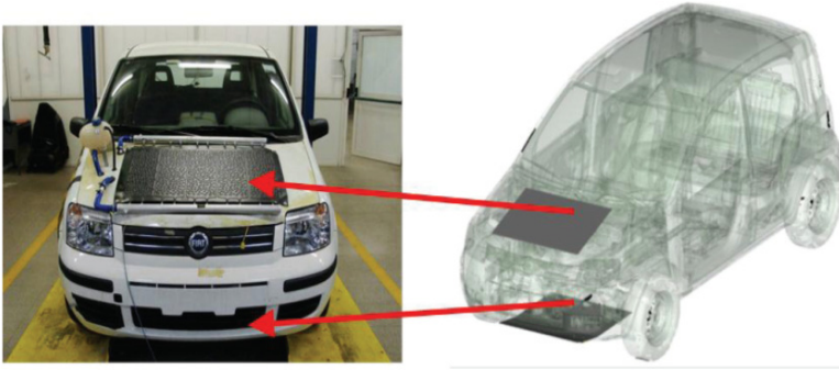
Fig. 2.3 Different positions of HEXs in a vehicle [18].
