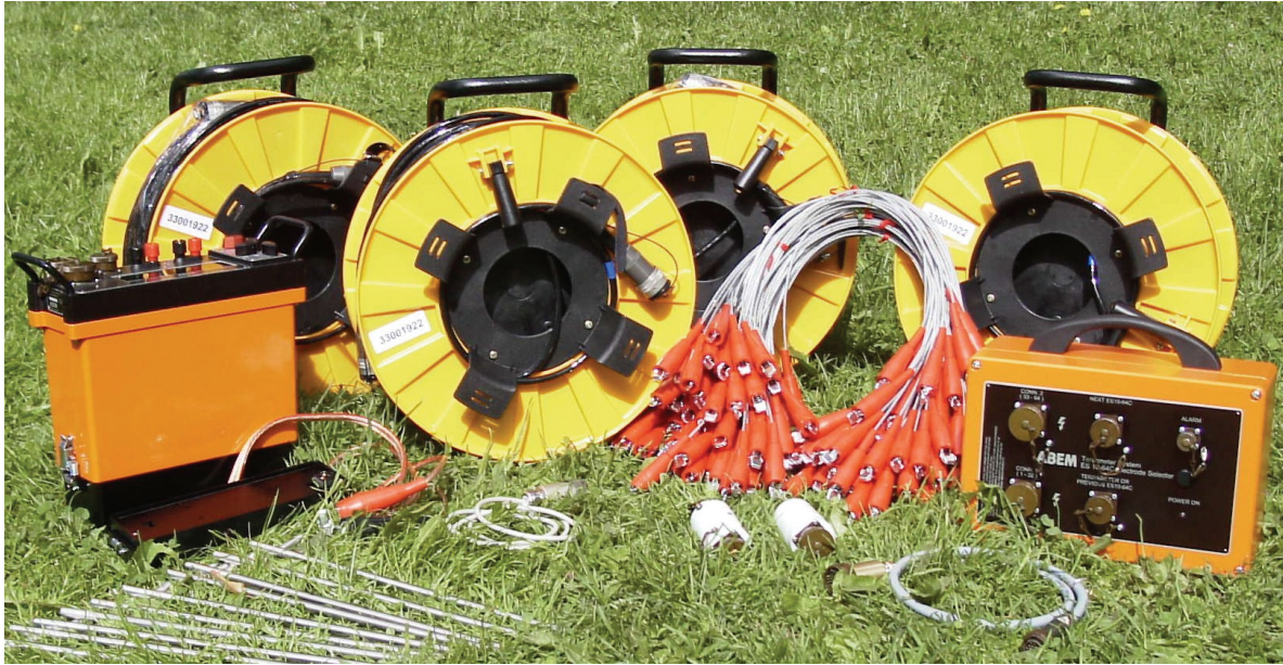
Figure 4-3 Picture showing an example of a commercially available data acquisition system, consisting of instrument, relay switch, electrode cables, stainless steel electrodes, cable jumpers and connection devices.
