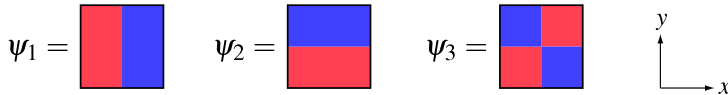
Figure 8: The two-dimensional Haar mother wavelet basis functions, \psi_M , are defined over the unit square with the values +1 where red, -1 where blue, and 0 elsewhere.
