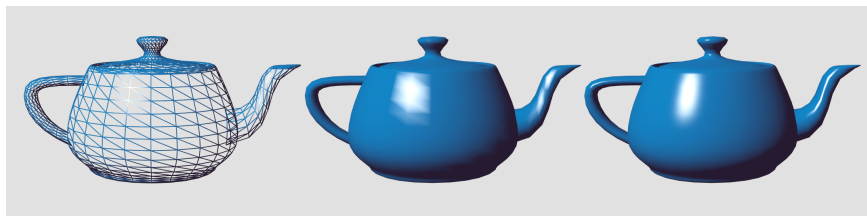
Figure 2: In the 1970s, it became possible to draw filled geometric primitives instead of just their outlines, as shown on the left. The different interpolation techniques that were developed, such as Gouraud (middle) [46] and Phong (right) [108] interpolation, were the first steps towards realistic shading.
