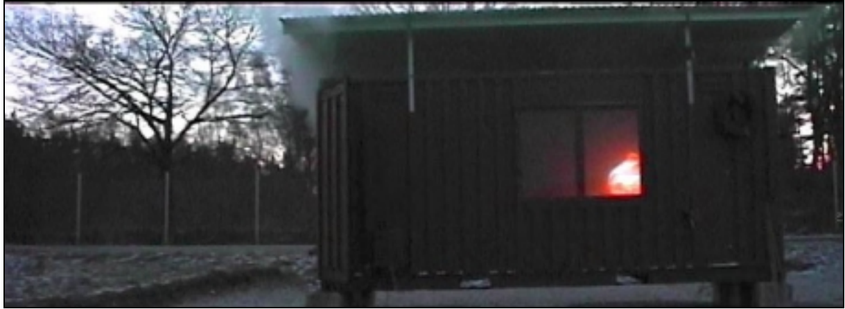
Figure 5. The gases inside the container are ignited.
