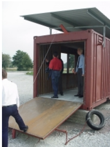
Figure 2. The pressure relief panel at its lowered position, making entry and exit to the container easier.
