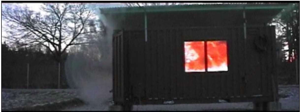
Figure 6. The heat generated causes a thermal expansion and the yet unburnt gases are expelled out of the container.
