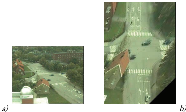
Figure 9. Rectification: a) the original image; b) the same image rectified. Note that the road plane is rectified nicely while objects above the road get more and more distorted the higher they appear (from Laureshyn & Ardö, 2006).
