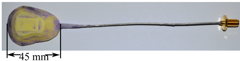
Figure 2.28: Top view of the fabricated encapsulated antenna. The yellow plastic is the casing in which epoxy-resin was filled. The semi-rigid feeding cable is also shown.
