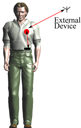
Figure 1.4: In-Body to On/Off Body Scenario where the circle represents an implant and the rectangle an on-body device.
