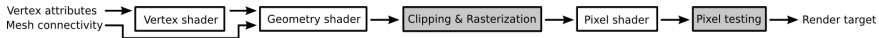
Figure 1: An overview of the pipeline of a modern GPU. White boxes represent the user-programmable stages and grey boxes represent fixed functionality.
