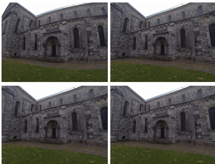
Figure 6.7: Example of corrected images based on the estimated \lambda by different solvers. Top left: Original image. Top right, bottom left and bottom right are images corrected according to 8-point, 7-point and 6-point one-sided method respectively.
