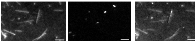
Figure 21 XUV image (left), IR image (middle) and XUV+IR image (right) of the same area. Scalebars are 10μm. The XUV and IR signals can have similar intensities.
