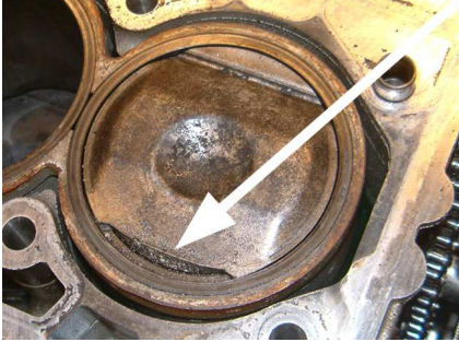
Figure 7: Damaged piston due to high PCP
