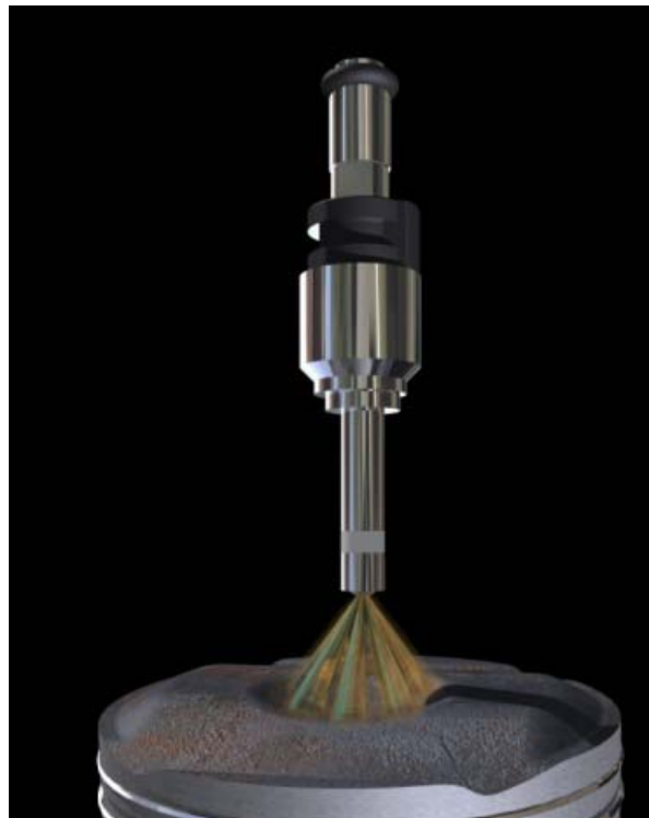
Figure 40: Fuel spray during the negative valve overlap
