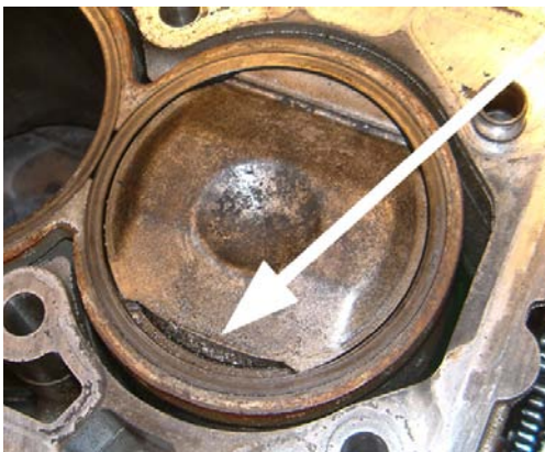
Figure 42: Damaged piston due to high PCP
