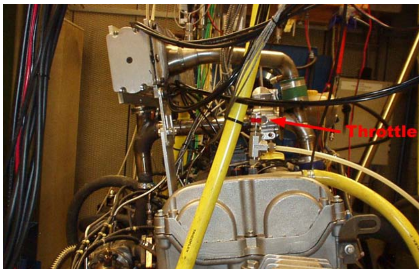
Figure 16: Throttle controlled intake temperature
