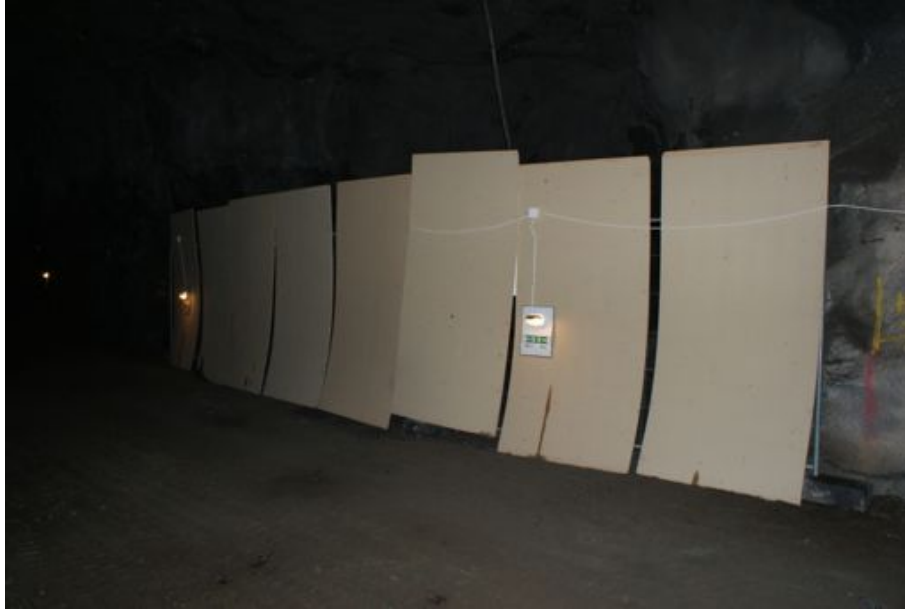
Figure 4. Sheets of particleboard were used to simulate the tunnel wall at one location in the tunnel.
