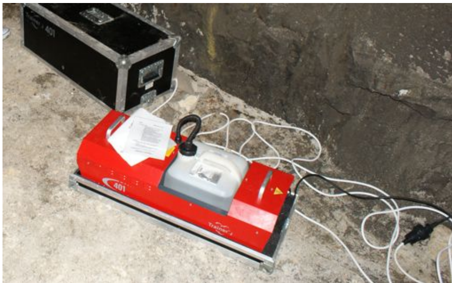
Figure 9. One of the smoke generators that were used to smoke-fill the tunnel in the experiment.
