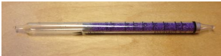
Figure 16. A test tube identical with the ones that was used to measure the gas concentration of acetic acid in the experiment.
