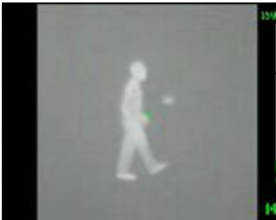
Figure 20. A snapshot from one of the video recordings of a participant walking in the tunnel. Just to the right of the participant, a light (installed on an emergency sign) is distinguishable as a small grey dot.
