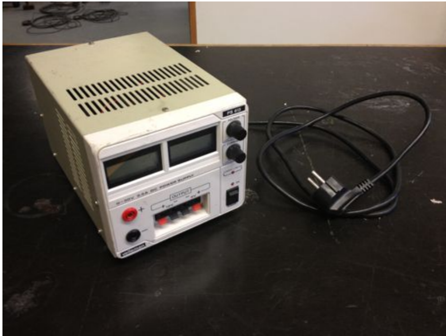
Figure 13. The power supply unit used in the experiment: a Velleman model PS-613.
