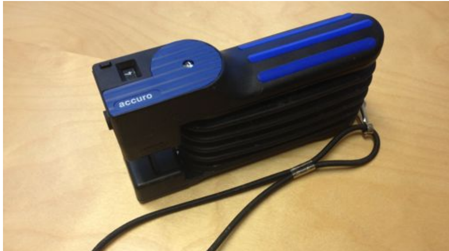
Figure 15. The gas pump used in the experiment to measure the gas concentration of acetic acid: an accuro Gas Detection Pump, manufactured by Dräger.
