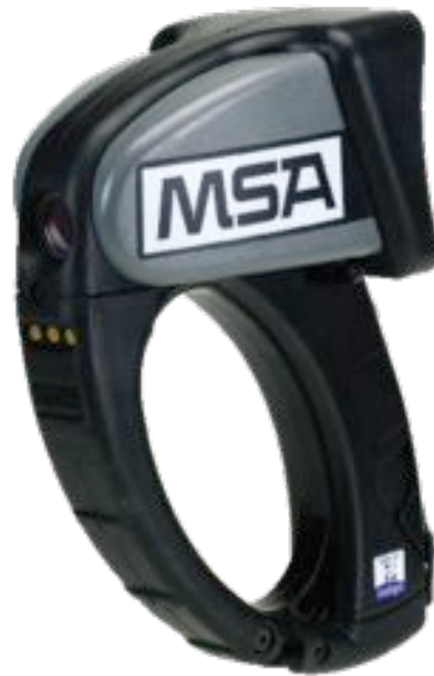
Figure 17. The thermal imaging camera used in the experiment: a MSA model Evolution 5600. Photo: MSA Nordic.
