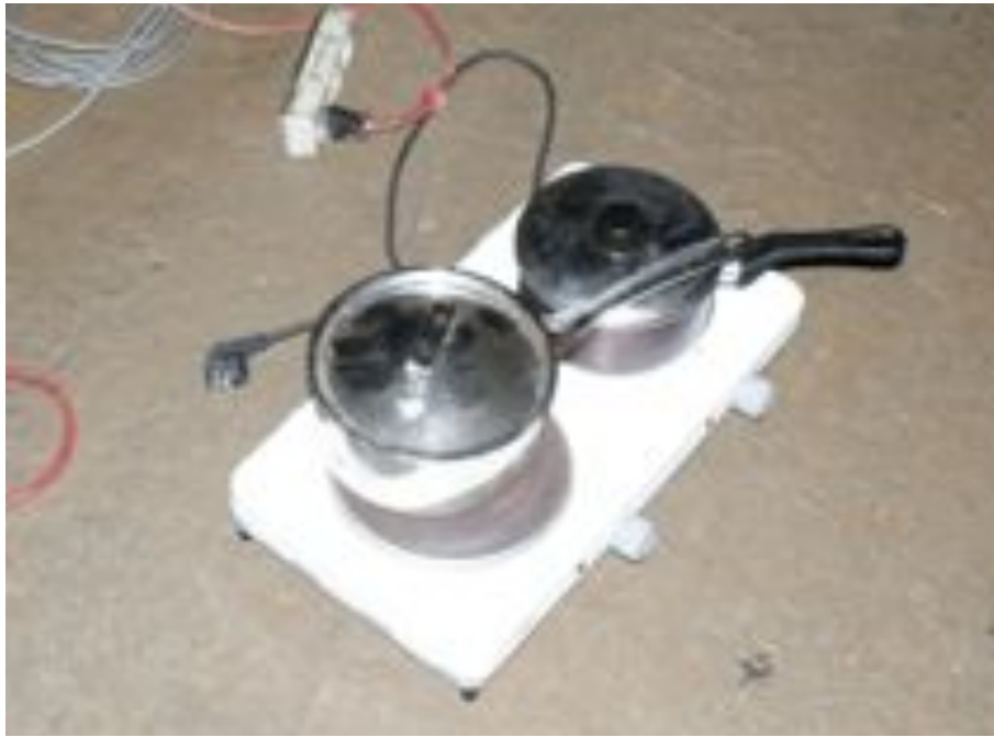
Figure 10. One of the mobile stoves, including pots, which were used to evaporate acetic acid in the experiment.
