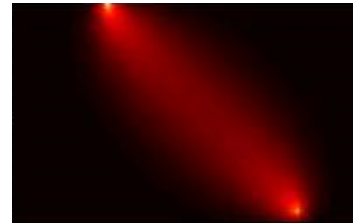
Figure 5.4. An example of the sensitivity profile between source and detector where regions with higher values will affect the measurement to a higher degree.
