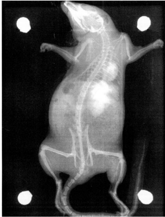
Figure 7. Image of a sacrificed Wistar-Furth rat, recorded on a normal radiographic imaging plate using a tantalum laser-produced x-ray source filtered by a thin copper sheet to cut off most of the radiation with energy below 25 keV (from [25]).
