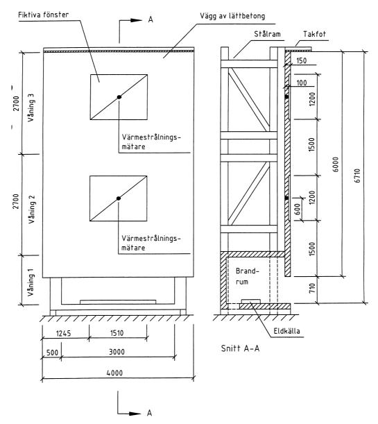
The SP-fire 105 test rig. From SP with permisson.
