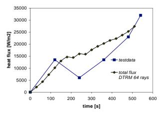
Figure 6.3 Comparison of predicted (from DTRM) and measured history of incident radiative heat flux to the lower fictious window.
