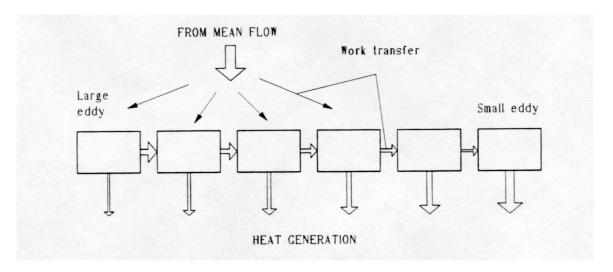
Figure 3.1 Turbulence energy transfer. [9]
