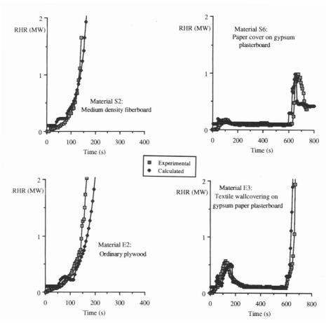
Figure 4.5 Comparison of calculated and measured heat release rates from the Room Corner test for 4 different surface lining materials (from [36]).
