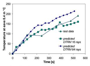
Figure 6.2 Comparison of predicted and measured temperatures at a distance 0.4 meters from facade under the eave. DTRM 64 rays.
