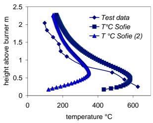
Figure 6.10 Gas-temperature distribution close to the calcium silicate board. Two predicted datasets from neighbouring vertical lines of control volumes in the simulation is presented illustrating the large gradients involved and the importance of precise knowledge of measurement positions.
