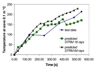
Figure 6.1 Comparison of predicted and measured temperatures at a distance 0.1 meters from facade under the eave.
