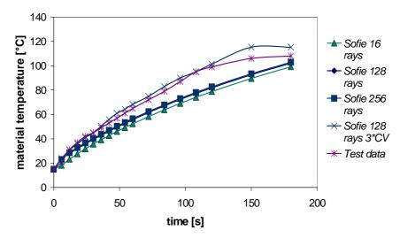
Figure 6.6 Material surface temperature time histories at about 1.1 meters above the burner. The difference in gas phase temperature is very small between simulations using the same mesh. For the finer mesh (using about 3 times the original set of control volumes) the temperature prediction is slightly more consistent with the experimental results.
