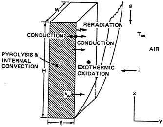
Figure 4.3 Schematics on heat transfer mechanisms. [23]
