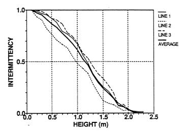
Figure 4.7. Flame height intermittence as function of vertical distance from the surface of the burner at a heat release rate of 300 kW. The different lines denote different locations relative to the centreline. [39]
