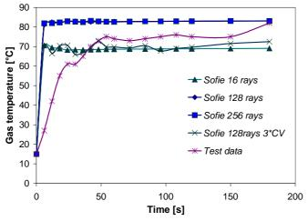
Figure 6.9 Gas temperatures 2.1 meters above the burner.
