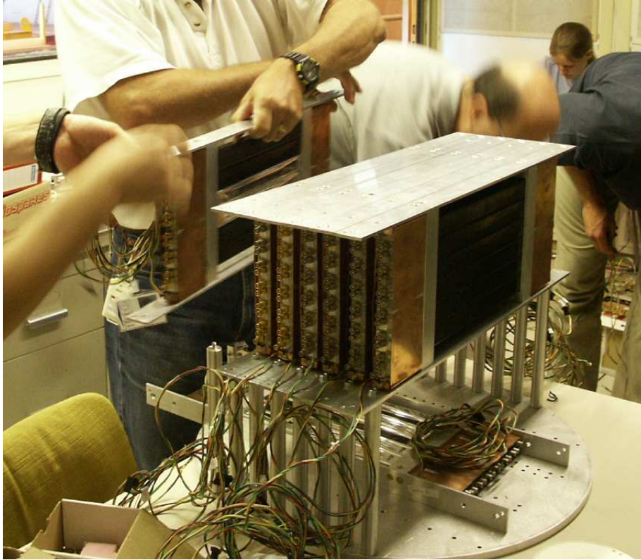
Figure 6.2: Assembling of the crystal layers onto the rotatable plate. The six CDEs of the first layer is clearly visible in black cover.
