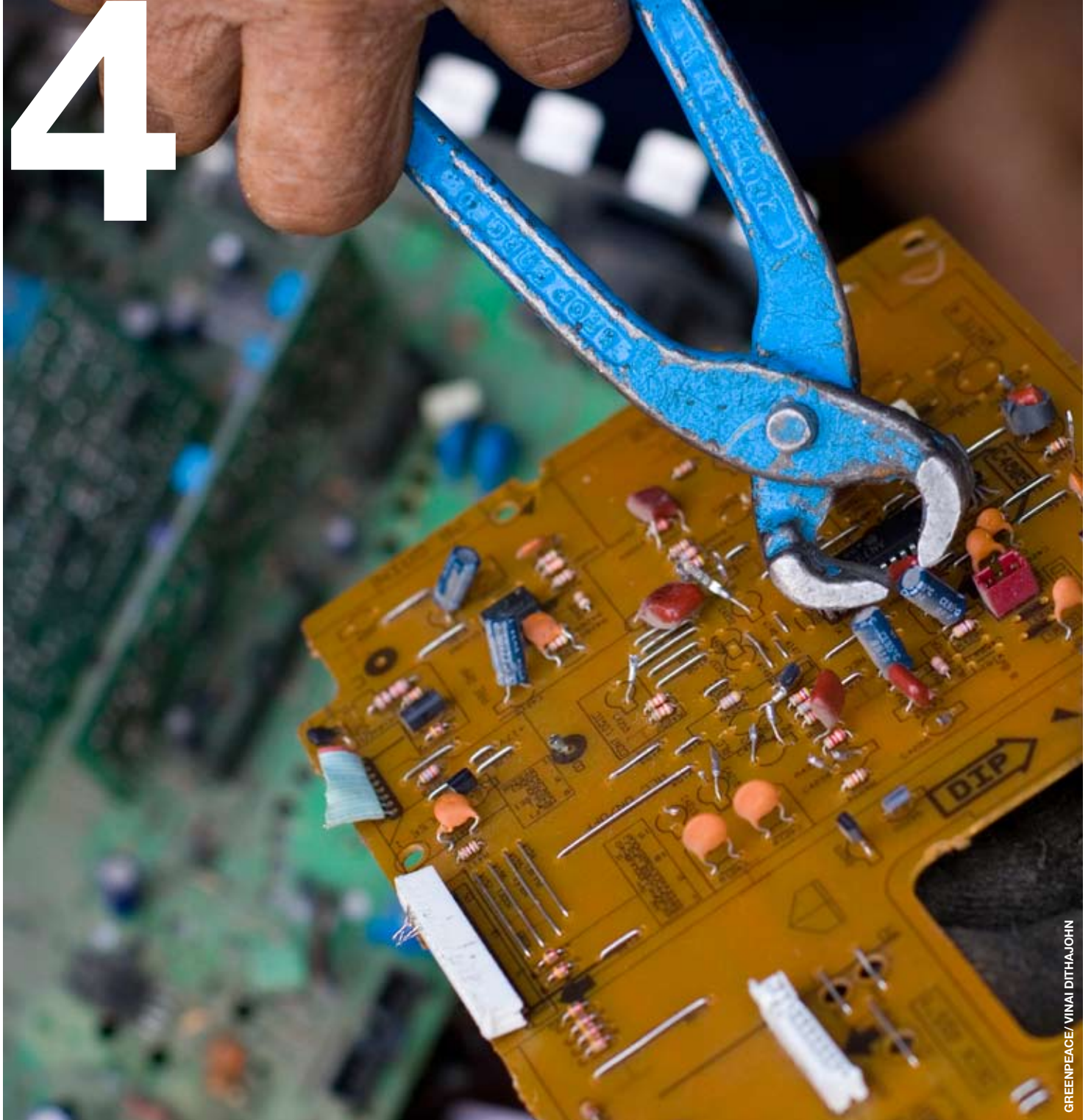
image Soi Suea Yai community, Bangkok - Printed wiring boards (PWBs) are dismantled by bare hand before being sold
