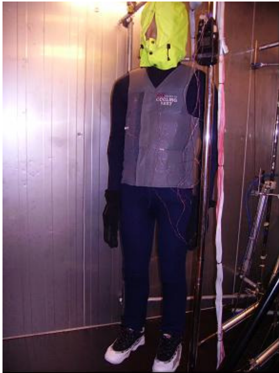
Fig. 1. The thermal manikin, clothing and PCM vest
