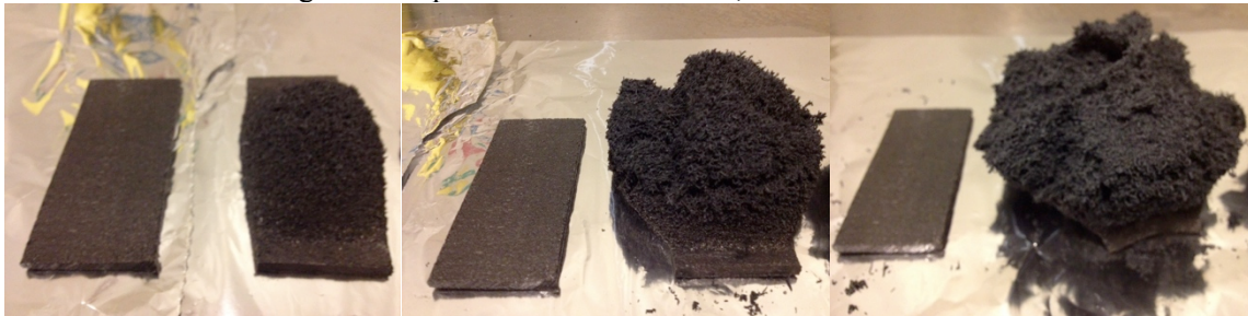
Figure 2: Expansion for test with 10, 15 and 20 \text{kW/m}^2 .
