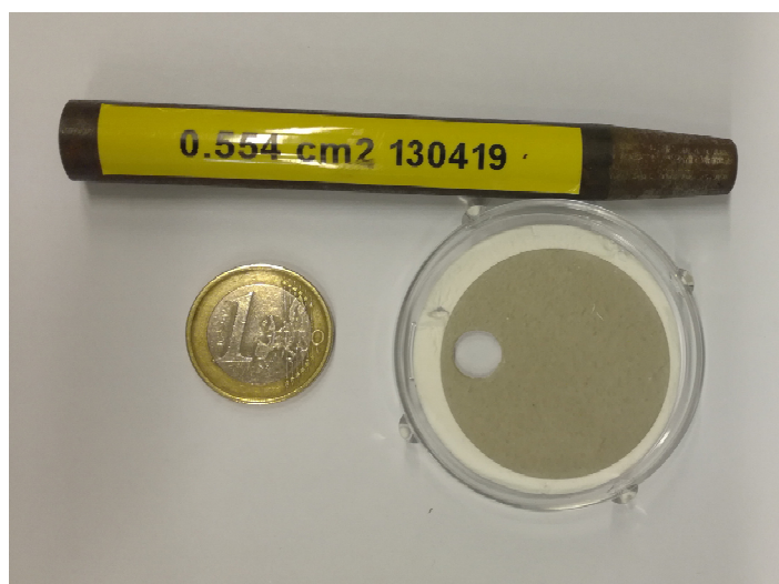
Figure 6. The picture shows an aerosol sample collected on 47 mm quartz-fibre filter. The darker circle on the filter represents the aerosol particle mass collected during sampling and the circular hole is a portion of filter punched out for analysis. The horizontal cylinder on top was the punch-cutter used to take sub-samples from the filter.
