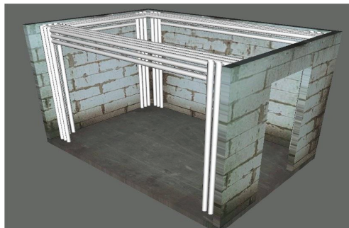
Figure 7. Schematic drawing of the pipe insulation installation in the Room Corner Test . The roof and left wall have been removed for better view. From ref [21].
