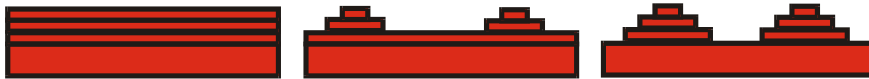
Fig. 6 Schematics of the three fundamental growth modes in hetero epitaxy. From the left: Frank Van der Merve growth mode, Stranski-Krastanow growth mode and Volmer-Weber growth mode
