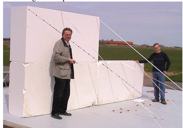
Figure 4. The authors in front of the three EPS blocks that were used to support the 25 coins. The coins were placed along the diagonal line. Note the plastic ties needed to keep the blocks in place.
