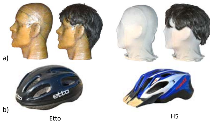
Figure 3. a) The head model as it is, with a wig and with a textile “skin” for “sweating” tests, and b) the tested helmets available on the market.
