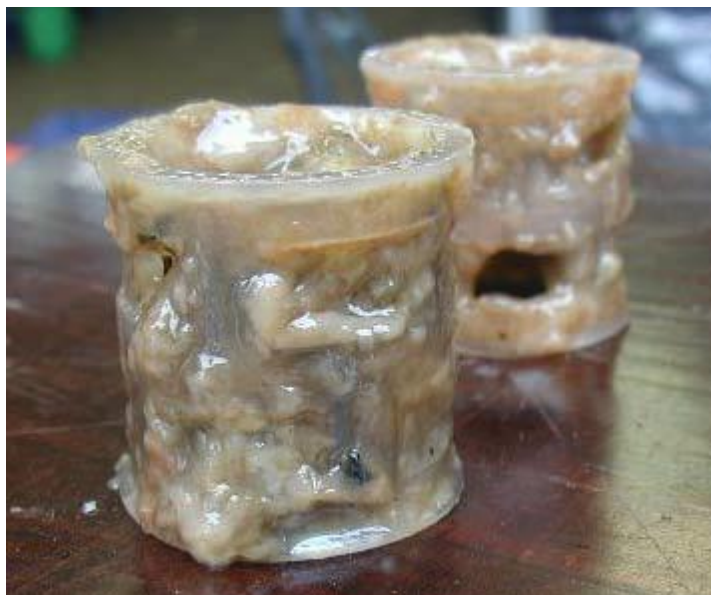
Figure 22 Microbial growth on pall rings used in water scrubber columns. Image from (Tynell 2005).
