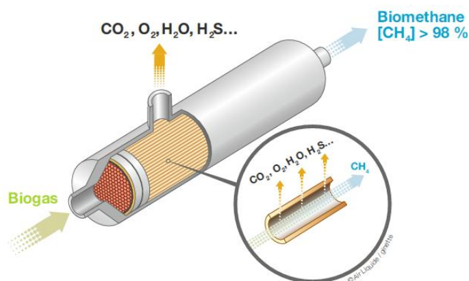
Figure 11 Illustration showing the separation involved during upgrading of biogas with membranes. Image from Air Liquide.
