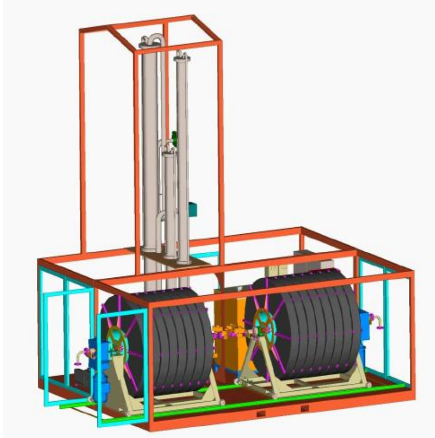
Figure 41 3D image of the Biosling upgrading unit with two rotating coils and a small water scrubber unit. Image from Biosling.
