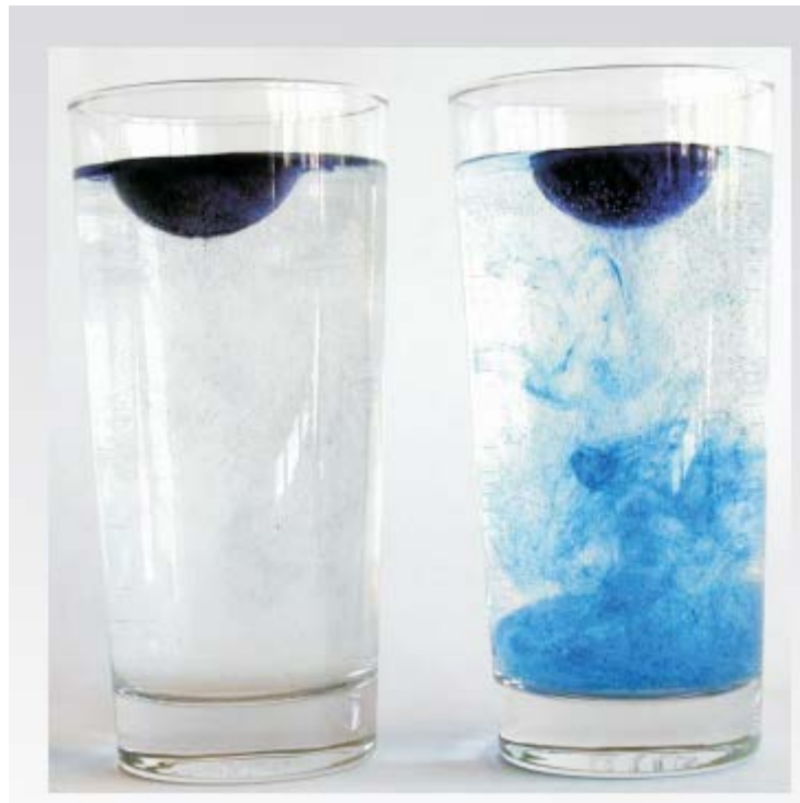
Figure 2. Ice cubes colored by food coloring. Left: salt water. Right: tap water.
