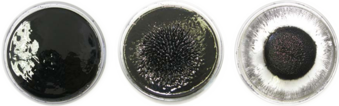
Figure 11. Homemade MR fluid in increasingly powerful magnetic fields
