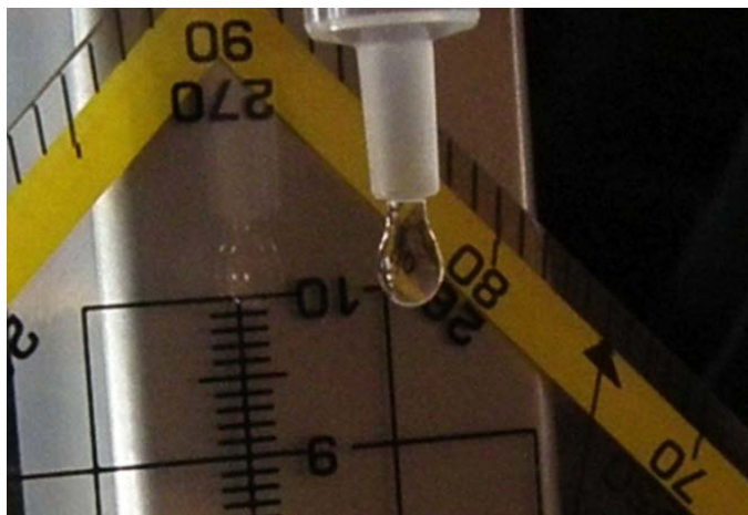
Figure 6. Measuring surface tension via the water drop
