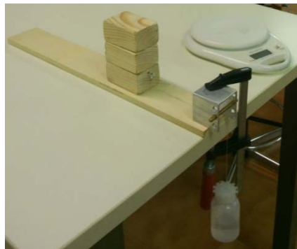
Figure 7. Wooden blocks could slide on a wooden plane. The experiment could be repeated with a different load, apparent area of contact or surface roughness.
