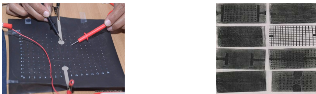
Figure 4. Designs for zero cost carbonized paper with electrodes to plot equipotential "surfaces"
