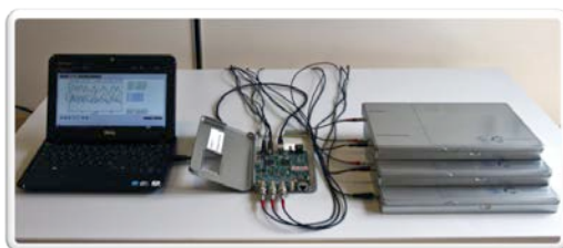
Figure 2. A set of the “CosMO” experiment with a notebook for the data analysis, a data acquisition card and three scintillator plates
