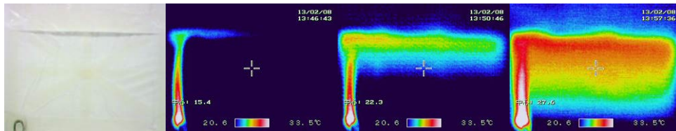
Figure 6. Another set of experimental results. In this case there is a heater at the left-bottom corner. These pictures clearly show that heat transfer in water differs from that which could be caused by convection.
