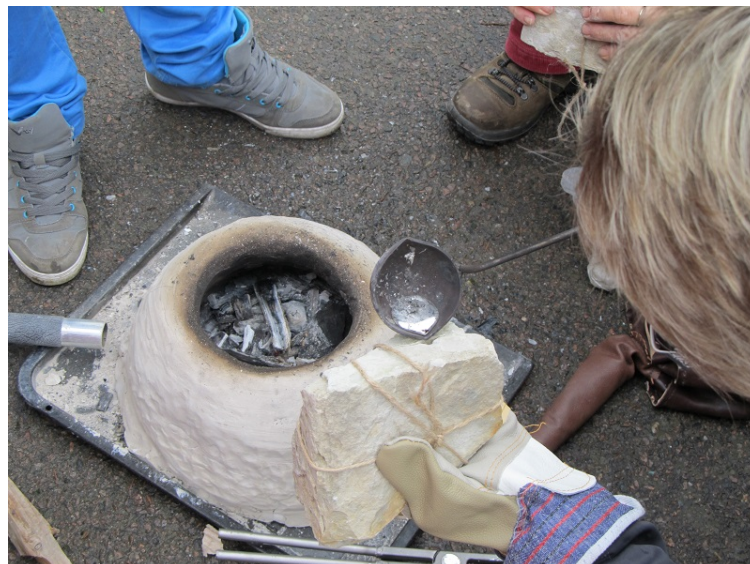
Figure 3. Tin casting in tufa
