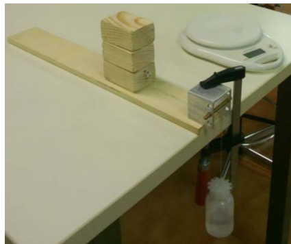
Figure 7. Wooden blocks could slide on a wooden plane. The experiment could be repeated with a different load, apparent area of contact or surface roughness.
