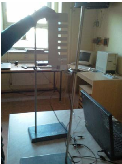
Figure 2. Free fall of a paper comb
