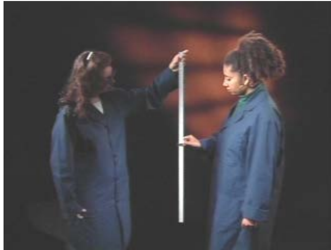
Figure 2. Example of a “tangible” to measure human reaction time. By dropping the meter stick from a fixed position, the time needed to catch the falling stick can be deduced by a direct measurement of the free-fall distance.
