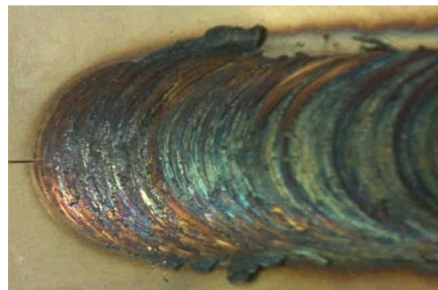
Figure 5: The weld without shielding gas showed severe oxidation during welding
