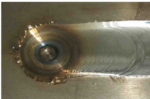
Figure 4: High quality FSW joints were obtained on the ESAB SuperStir™ machine
