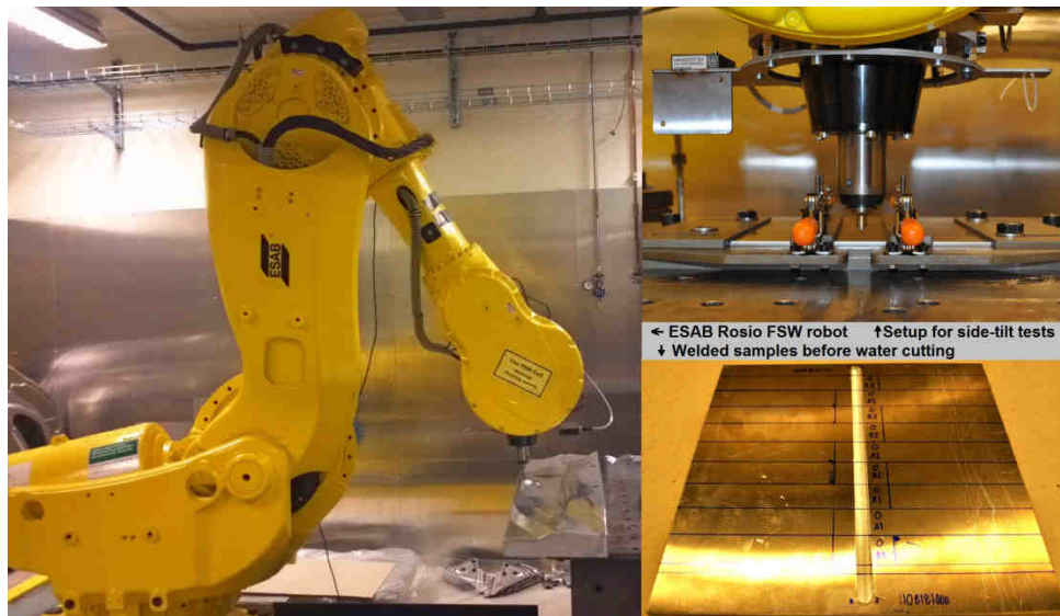
Figure 1: FSW robot at the Production Technology Centre (left) and the experimental set-up (right)
