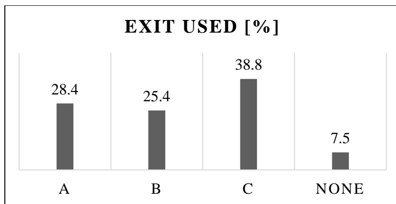
Figure 17. Proportion of participants using the different exits. Exit C was the closest to the fire.
