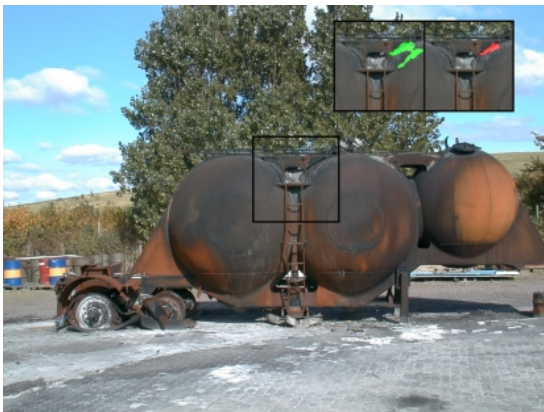
Fig. C4. A burned-out gas tank provides the backdrop for imaging pollutant gas leaks. Green pixels highlight areas where ammonia and ethylene gases are leaking. Red shows the selective detection of ammonia with a gas correlation cell.
