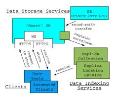
Figure 1: Interaction between the SSE and other components.
