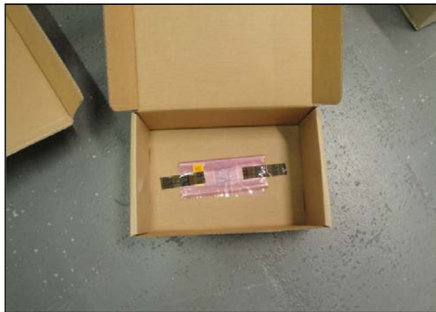
Figure 9. Example of low fill rate. Product attached to the bottom of the box
