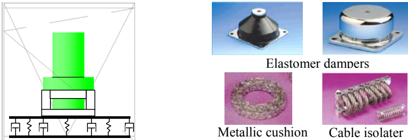
Figure 5. Presentation of the concept with a transportation pallet working principle
