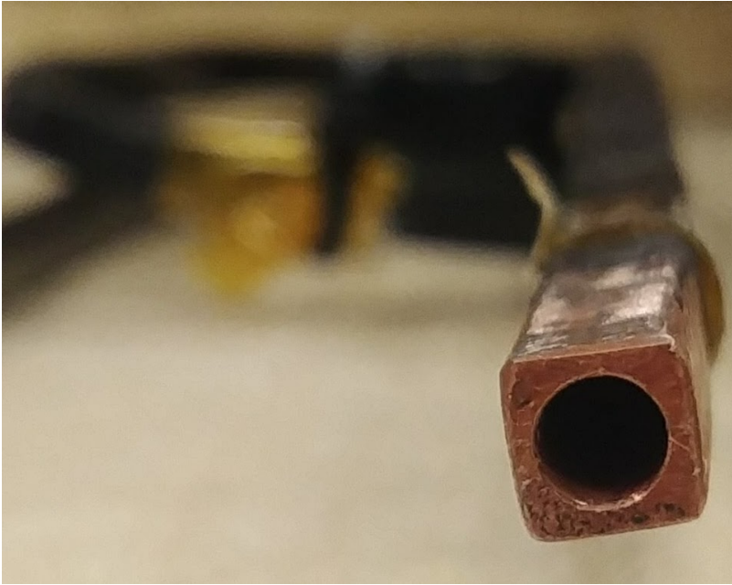
Figure 3.10: Photo of a 6x6 mm rectangular hollow winding with 2 mm radius inner air channel.
