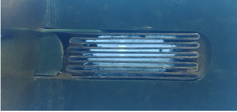
Figure 3.8: Example of folded laminated winding with relatively even spaces for air flow.
