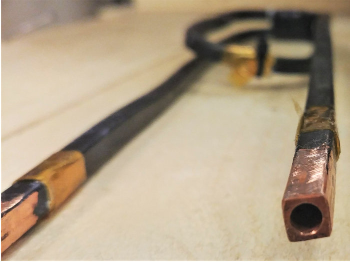
Figure 4.8: Photo of outlet cross section of copper conductor used for experiment.
