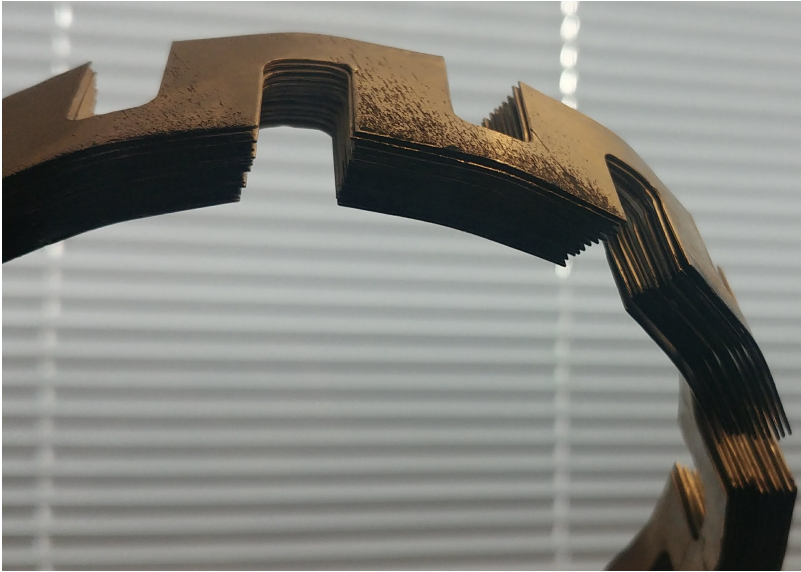
Figure 3.5: Example of rolled laminated winding for a machine with a short active length.
