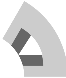
Figure 3.3: Illustration of section of SRM stator with a triangular cooling "prism" between the windings.
