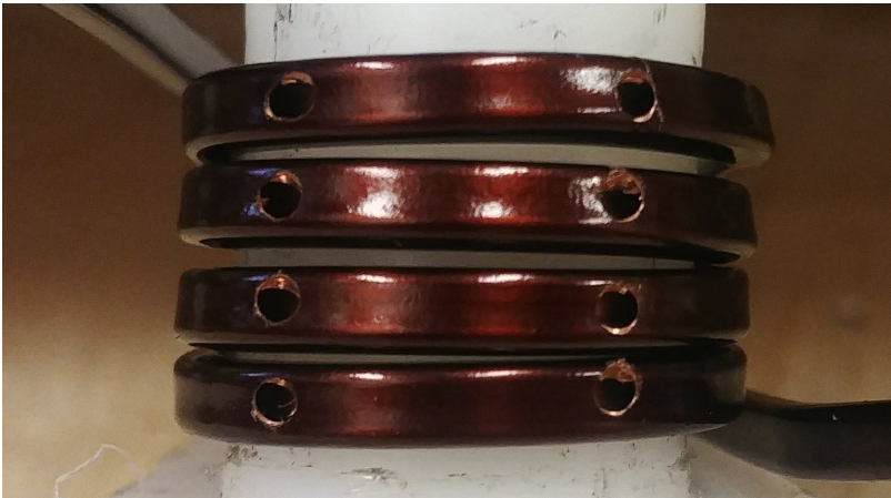
Figure 3.12: Close-up photo of end windings of coiled hollow rectangular winding with drilled holes for parallel air inlets/outlets.
