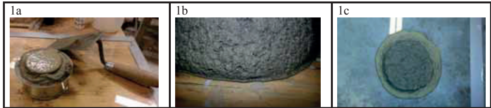
Figure 1. 1a) The Hägermann cone filled with mortar. 1b) When the edge of a mortar is considered to indicate no risk for water separation according to the grading system. 1c) A combination with clear risk for water separation, which happened before the mortar acquired an acceptable workability.
