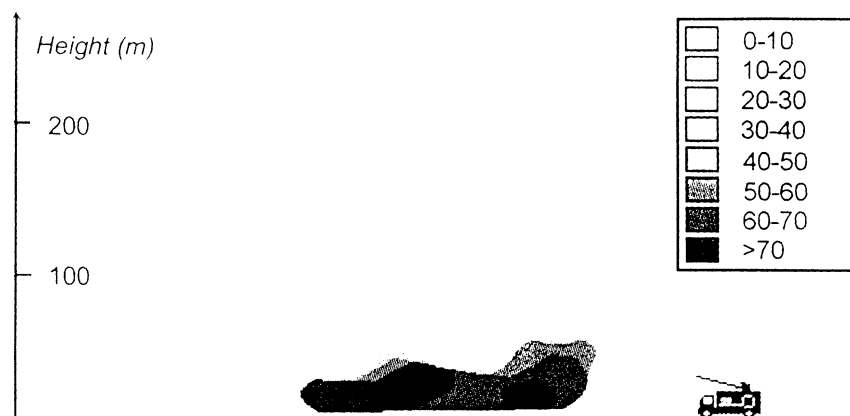
Fig. 3. Results from measurements of NO along a street in Prague, showing increased concentrations at two subsequent street crossings. Concentration values are given in \mu\text{g}/\text{m}^3 . (Adapted from Engst et al. 1995).
