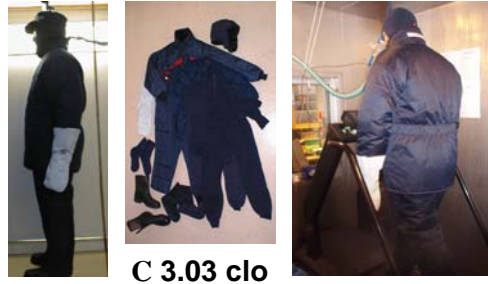
Figure 1. Ensemble C of Subzero project on manikin, as items and on a subject.
