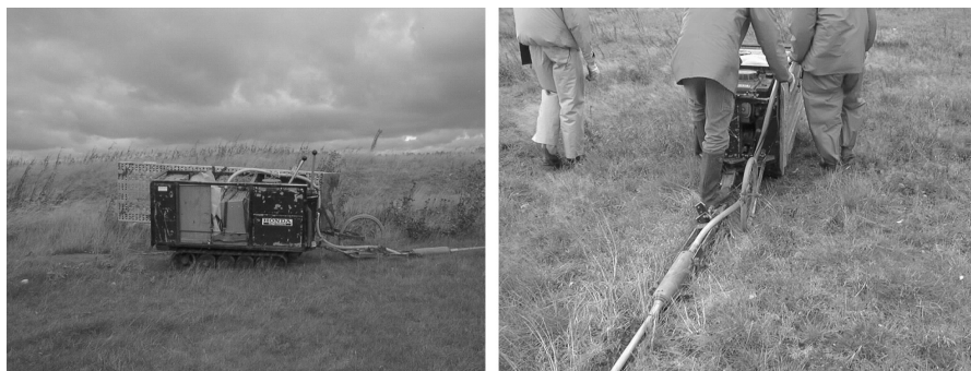
Figure 8 Photograph of the PACES system. (left) The small caterpillar seen from the side. A portable bridge is mounted on one side and the electrode streamer is visible behind the caterpillar. Note the wheel that measures travelled distance. (right) The operator standing on a small plough mounted just behind the caterpillar for improvement of the electrodes contact with the ground. The cylinder mounted on the cable just behind the plough is the first electrode.
