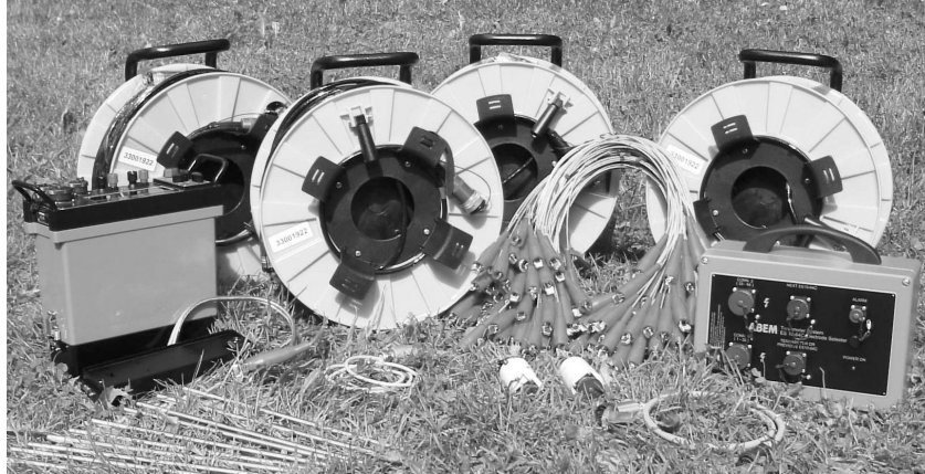
Figure 7 Photograph of one version of the ABEM Lund Imaging System including the instrument SAS4000, an electrode selector ES-1064, multi-conductor cables, electrodes, a battery and various connectors.
