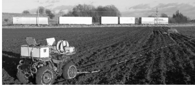
Figure 16 Photographs of the land-streamer and 4WD. Note the Geometrics Geode mounted on the rear of the 4WD.
