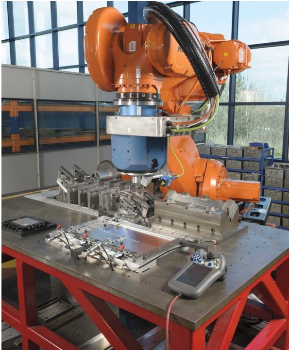
Fig. 2. Overview of the robot cell and the ABB IRB 7600 robot arm with 6 DOF used in the experiments.
