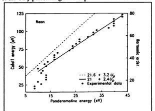
Fig. 1 Cutoff energy in neon as a function of the ponderomotive energy. The solid line is a linear best fit: 21+2.4 Up, the dashed line is the prediction of the single-atom response 21.6+3.2 Up. From Ref 6.
