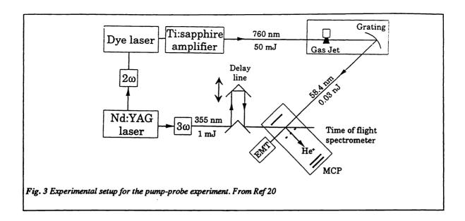
This experiment demonstrates that the high-order harmonics can be used for two-color pump-probe experiments. It enables cascade-free studies of radiative properties of atomic and ionic systems in the XUV spectral range. Note that it is possible to go to much shorter wavelengths and shorter pulse durations than those used in the present experiment, by using a pump laser with a shorter pulse duration. This could be useful for measurements of very short radiative processes.
