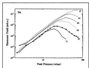
FIG 2 Number of photons at different harmonic frequencies (from the 57th, in the plateau to the 71st, last visible harmonic) as a function of atomic pressure. The laser used was a 150 fs Ti:S system. From Ref 12.
