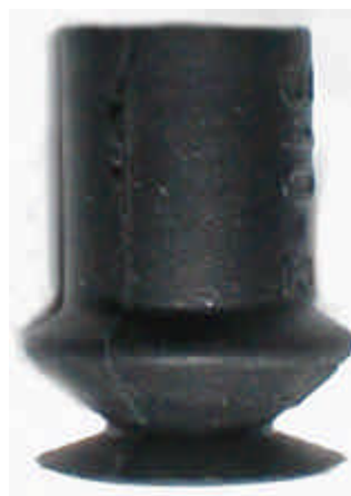
Figure 4.13 A bellow-type suction cup is used for page separation.
