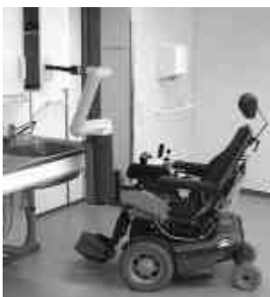
Figure 5.5 The Manus arm mounted on a Permobil Max90 wheelchair.
