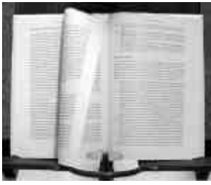
Figure 4.38 By moving the upper corner of the page downwards at the end of the turning movement, the lower corner of the page is moved to the left, making room for the finger of the readerboard.
