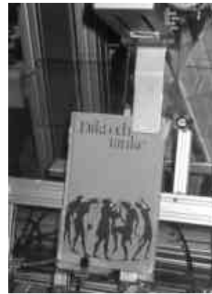
Figure 4.49 The page turning gripper is designed to open books from the same position regardless of the size of the book.
