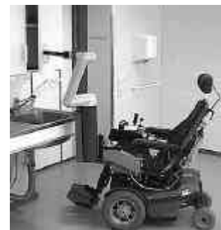
Figure 1.2 The wheelchair-mounted Manus manipulator opening a kitchen cupboard.
