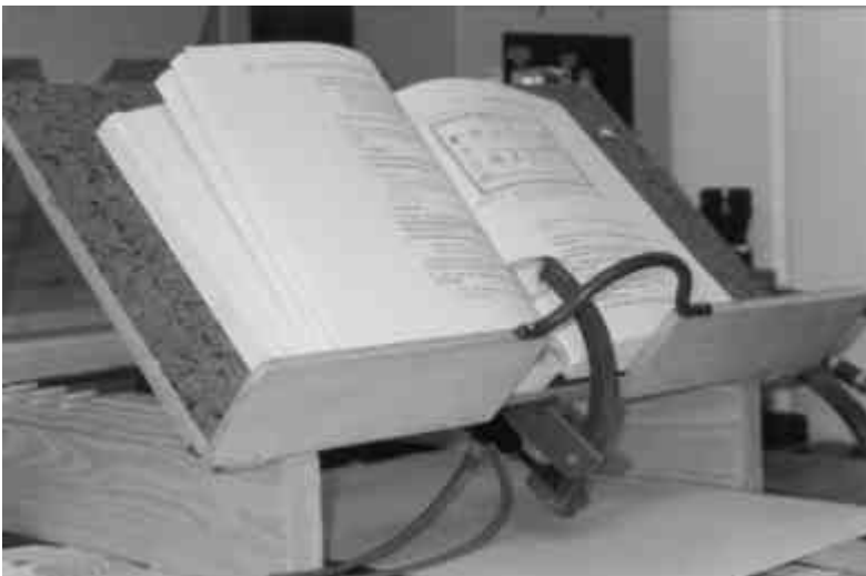
Figure 4.21 A prototype of the RAID1 readerboard. The readerboard has functions which facilitate turning the pages of books.
