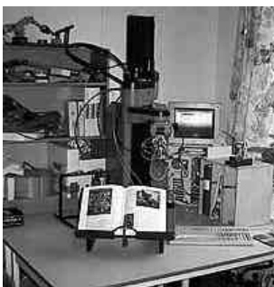
Figure 4.26 An RT100 robot was used for testing the end-effector prototypes developed for RAID1.
