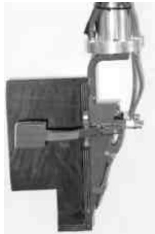
Figure 4.24 A prototype of the RAID1 book gripper.
