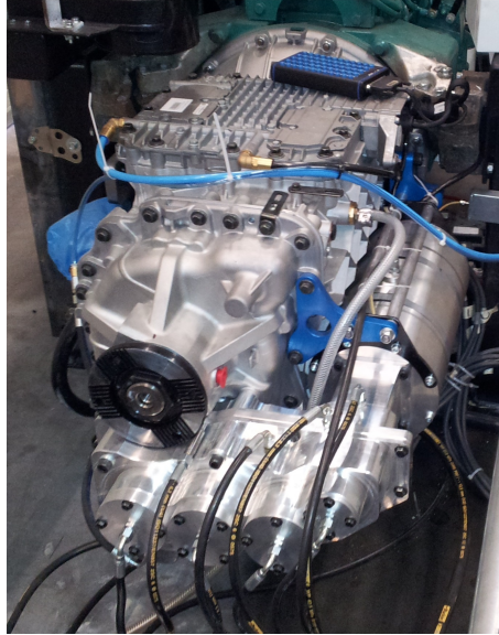
Figure 2.18: The prototype machine mounted at the side of the AMT-gearbox in the system test rig
