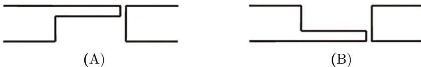
Figure 4.1: Schematic drawing of the limitations of negative UV-resists. (A) It is not possible to directly cross-link a free-hanging cantilever on top of its chip body. (B) Therefore, cantilever chips need to be fabricated up-side-down.
