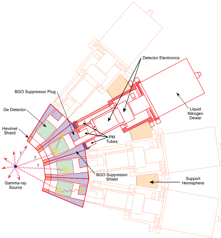
Figure 2.2: Ge detectors in the Gammasphere array [25]. Picture taken from [23].
