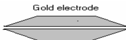
Figure 11. The gold capillary working electrode of the spectroelectrochemical set-up.
