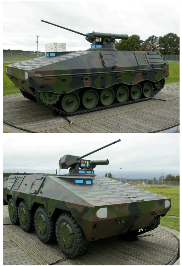
Fig. 8. The STANDCAM test target. The right side is wheeled and the left side is tracked.
