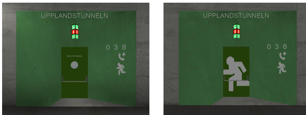
Figure 2. Exemplary representation of the VR emergency exit portal in presence of a window (left) or a running man (right) on the door.
